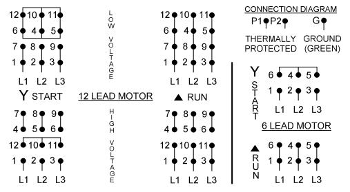
FULL VOLTAGE ACROSS THE LINE START AND RUN ON  $\triangle$  CONNECTION. ALSO SUITABLE FOR START ON Y, RUN ON  $\triangle$ .
